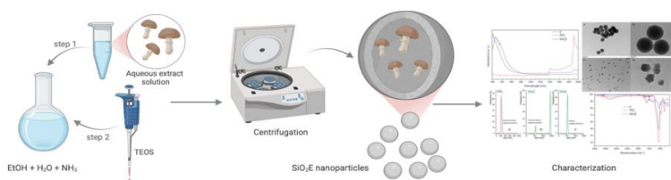
Figure 1. Schematic illustration of SiO 2 NP s nanoparticle synthesis and characterization
