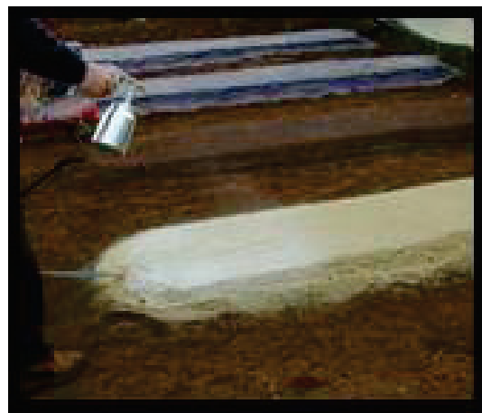
Figure 2. Spray application of a neutral polysaccharide based film on a bed of pulverized fibers
