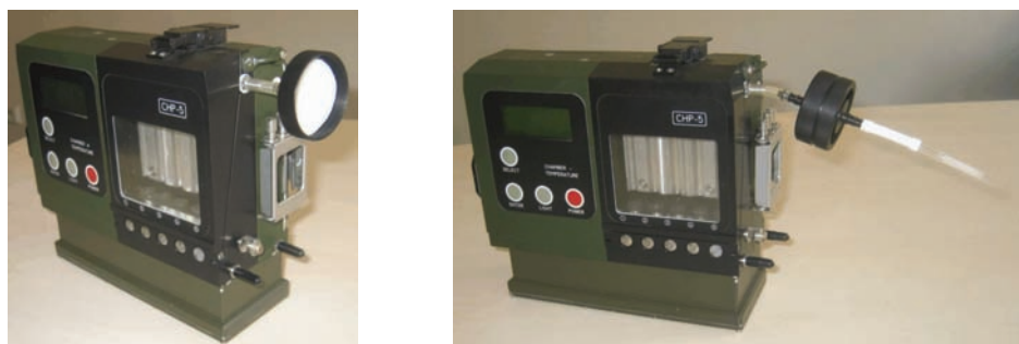
Fig. 2. Apparatus photo: CHP-5 with indicator disc and adapter (a); CHP-5 with indicator disc, chlorinating cartridge and adapter (b).
