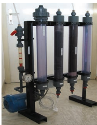
Fig. 1. Laboratory equipment for arsenic removal with \alpha\text{-FeOOH} (TA) filter media.
