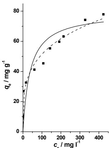
Fig. 4. Sorption isotherm of phosphate on  $MgZn_2Al$  hydrotalcite.
