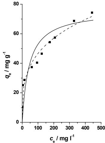
Fig. 5. Sorption isotherm of phosphate on  $Zn_3Al$  hydrotalcite.
