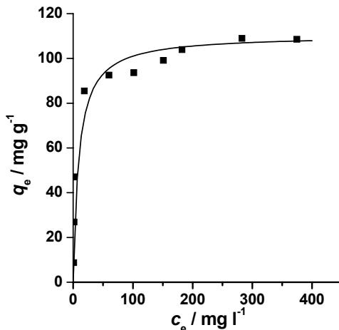
Fig. 1. Sorption isotherm of phosphate on Mg<sub>3</sub>Al hydrotalcite.
