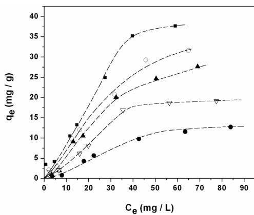
Fig. 6. Sorption isotherms for thiocyanate on:  $Mg_3Al$  (■);  $Mg_2ZnAl$  (○);  $Mg_{1.5}Zn_{1.5}Al$  (▲);  $MgZn_2Al$  (▽);  $Zn_3Al$  (●). Lines are drawn to guide the eye.
