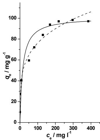
Fig. 2. Sorption isotherm of phosphate on  $Mg_2ZnAl$  hydrotalcite: full line – Langmuir isotherm; dotted line – Freundlich isotherm.
