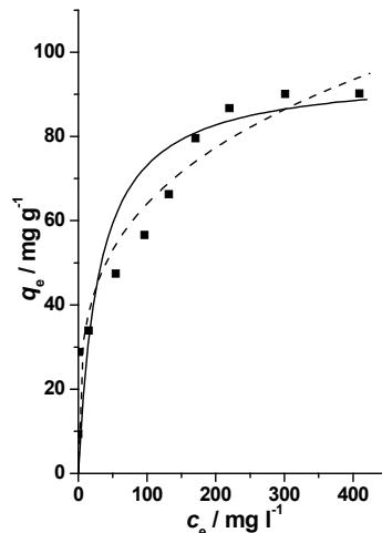
Fig. 3. Sorption isotherm of phosphate on  $Mg_{1.5}Zn_{1.5}Al$  hydrotalcite.
