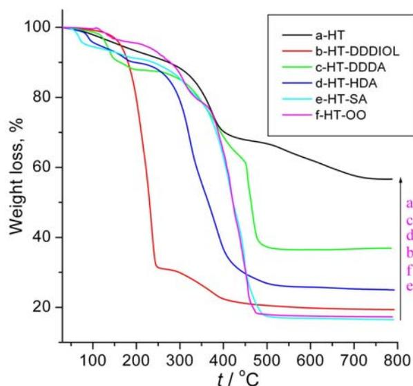
Fig. 3. TGA of a) HT, b) HT–DDDIOL, c) HT–DDDA, d) HT–HDA, e) HT–SA and f) HT–OO.
