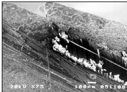
Fig. 4. SEM Micrograph of the cracking of outer layer of specimen subjected to impact load on enlargement \times 75 ; test sample I-D-1.
