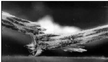
Fig. 6. Delaminations between layers in test sample I-C-2.
