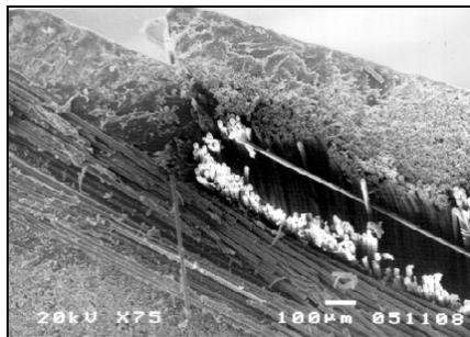
Fig. 4. SEM Micrograph of the cracking of outer layer of specimen subjected to impact load on enlargement  $\times 75$ ; test sample I-D-1.
