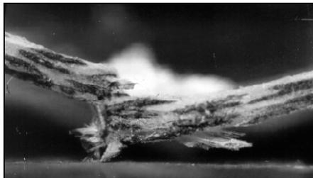
Fig. 6. Delaminations between layers in test sample I-C-2.
