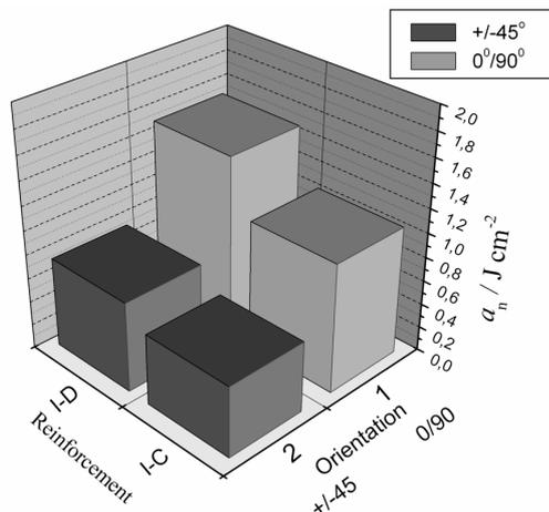
Fig. 2. Impact strength, average values at 20 °C.
