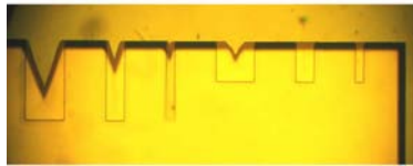
Fig. 3. OM Photographs of the microcantilevers undercut process in 25 wt. % TMAH solution on (100) Si wafers when the etching time was 0.75 h (top) and 1.25 h (bottom). The microcantilevers were oriented in the \langle 110 \rangle direction.
