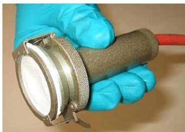
Fig. 1. Filter with adapter.
