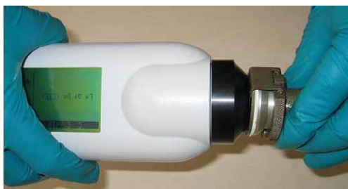
Fig. 2. Measurement of filter coloration by tristimulus colorimeter.
