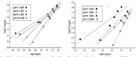
Fig. 3. Freundlich adsorption isotherm of LABS on Fig. 4. Freundlich adsorption isotherm of DBS on acactive carbon at different pH. tive carbon at different pH.
