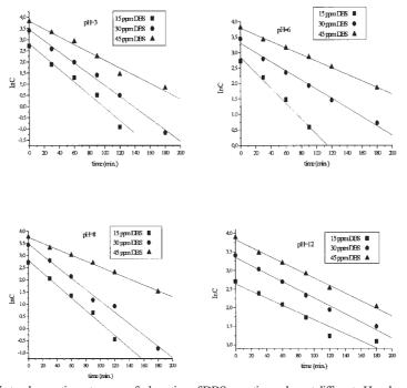
Fig. 2. The first order reaction rate curve of adsorption of DBS on active carbon at different pH and concentrations.
