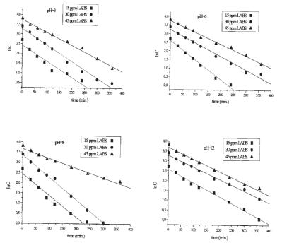
Fig. 1. The first order reaction rate curve of adsorption of LABS on active carbon at different pH and concentrations.
