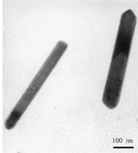
Fig. 2. Morphologies of two as-prepared Cu nanorods obtained at a constant current of  $0.14 \text{ mA cm}^{-2}$  for 30 min.
