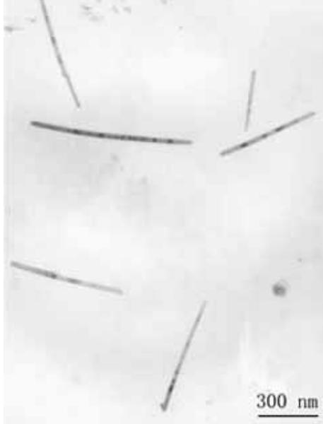
Fig. 1. TEM images of Cu nanorods obtained at a constant current of  $0.14 \text{ mA cm}^{-2}$  for 30 min. Mean diameter 30 nm. Mean length 500 nm.
