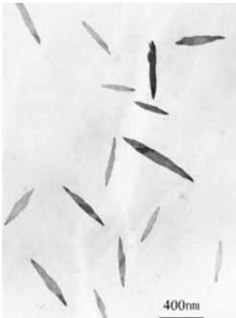
Fig. 3. TEM images of CuI nanorods obtained at a constant current of  $0.3 \text{ mA cm}^{-2}$  for 30 min.
