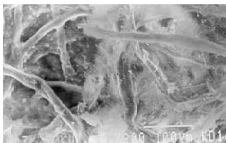
Fig. 1. SEM of the sepiolite – cellulose paper (60 % : 40 %).
