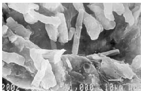
Fig. 2. SEM of crystallized \text{NH}_4\text{NO}_3 in the sepiolite paper.
