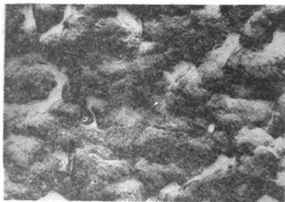
Fig. 4. \text{Na}_2\text{CO}_3 surface (magnified 47000 \times )
