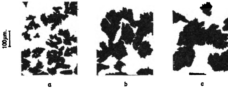
Fig. 3. Copper powders obtained by pulsating overpotentials of different shapes: (a) square-wave, (b) sinusoidal, (c) triangular. Overpotential amplitude 700 mV. Frequency of pulsation 100 Hz.
