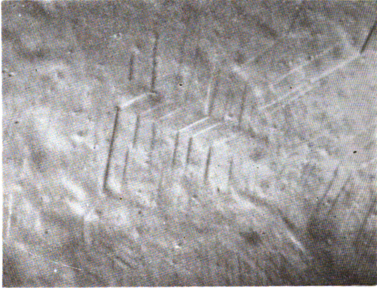
Fig. 4 Copper, microstructure after 1 cycle; interference contrast
