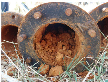
Fig. 2. Encrustations in a discharge pipe of Well Bn-6 at the water supply source of Trnovče (picture taken on 1 Sep, 2011).
