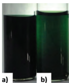
Fig. 5. Photographs of solutions of PANI-PIA in mixtures, a) water/THF = 0.428 and b) water/NMP = 0.428.
