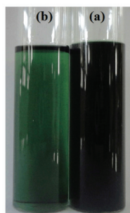
Fig. 5. Digital photos of solutions of: a) concentrated and b) dilute solution of PANI-IAs in DMSO solvent.
