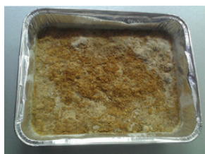
Fig. 1. SSF appearance on the tray after 36 h.
