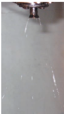
Fig. 2. Melt electrospinning with an umbrella-like spray head.
