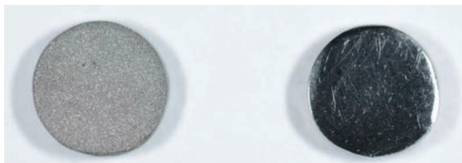
Fig. 1. CM Samples (left – cast and sandblasted, right – polished).
