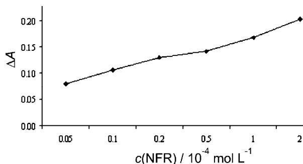
Fig. 2. Effect of the nuclear fast red concentration on  $\Delta A$ . Conditions:  $10\text{ }\mu\text{g mL}^{-1}$  nitrite;  $0.20\text{ mol L}^{-1}$  sulfuric acid;  $0.020\text{ mol L}^{-1}$  potassium bromate; temperature:  $25\text{ }^{\circ}\text{C}$ ; reaction time: 5 min.
