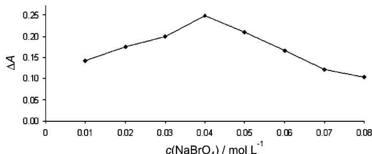
Fig. 3. Effect of the potassium bromate concentration on  $\Delta A$ . Conditions:  $10 \mu\text{g mL}^{-1}$  nitrite;  $0.20 \text{ mol L}^{-1}$  sulfuric acid;  $1.0 \times 10^{-4} \text{ mol L}^{-1}$  nuclear fast red, temperature:  $25^\circ\text{C}$ ; reaction time: 5 min
