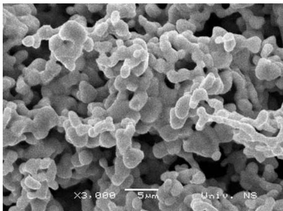
Fig. 7. An SEM microphotograph of the  $\text{Sb}_2\text{Co}$  alloy.
