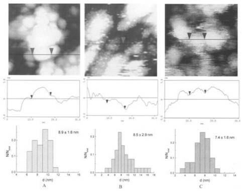
Fig. 2. STM Images of GC–C/Pt (polished support – A), GC–G<sub>OX-AL</sub>/Pt (GC support oxidized at 1.41 V vs. SCE for 95 s – B) and GC-G<sub>OX-AC</sub>/Pt (GC support oxidized at 2.25 V vs. SCE for 95 s – C)  $w_{Pt} = 18 \pm 1 \ \mu g/cm^2$ .
