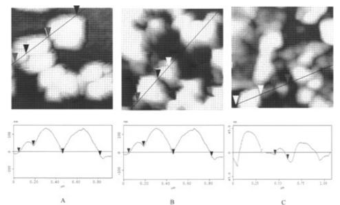
Fig. 1. AFM Images of GC–G/Pt (polisher support – A), GC–G<sub>OX-AL</sub>/Pt (GC support oxidized at 1.41 V vs SCE for 95 s –B) and GC–G<sub>OX-AC</sub>/Pt (GC support oxidized at 2.25 V vs. SCE for 95 s – C)  $w_{Pt} = 18 \pm 1 \ \mu g/cm^2$ .
