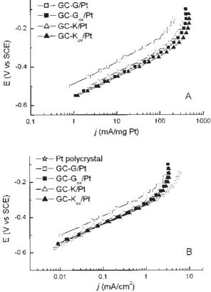
Fig. 5. Steady state polurization curves for the oxidation of 0.5 M CH<sub>3</sub>OH in 0.1 M NaOH at GC/Pt with polished supports and GC<sub>OX-AL</sub>/Pt with oxidized supports. ( $w_{Pt} = 18 \pm 1 \ \mu g/cm^2$ , GC supports oxidized at 1.41 V vs. SCE for 95 s, sweep rate 1 mV/s; A–mass activity and B–specific activity scale).
