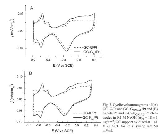
of the voltammograms for  $GC_{OX-AC}/Pt$  electrodes with a support previously oxidized in acidic solution strongly depend on the time and potential of the anodic polarization of the glassy carbon. Hence, if GC is oxidized at the same potential but for a shorter time, the CV for  $GC_{OX}/Pt$  reveals the presence of characteristic peaks for both Pt and oxidized glassy carbon.<sup>24</sup>
