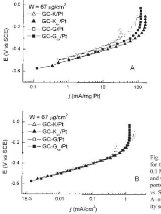
Fig. 6. Steady state polarization curves for the oxidation of 0.5 M CH<sub>3</sub>OH in 0.1 M NaOH at Pt deposited on GC–G and GC–K polished and oxidized supports (GC support oxidized at 1.41 V vs. SCE for 95 s;  $w_{Pt} = 67 \pm 2 \ \mu g/cm^2$ ; A–mass activity and B–specific activity scale).
