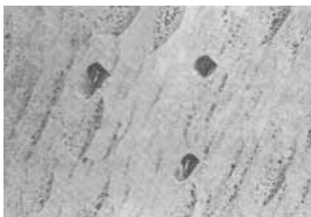
Fig. 2. A view of an etched (001) cleavage plane of a Nd:CaWO 4 single crystal plate after an etching exposure time of 30 min. Dislocation density 638 cm -2 . Magnification 270×.
