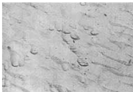
Fig. 3. A view of an etched (001) cleavage plane of a Nd:CaWO 4 single crystal plate after an etching exposure time of 15 min. Dislocation density 3200 cm -2 . Magnification 270×.
