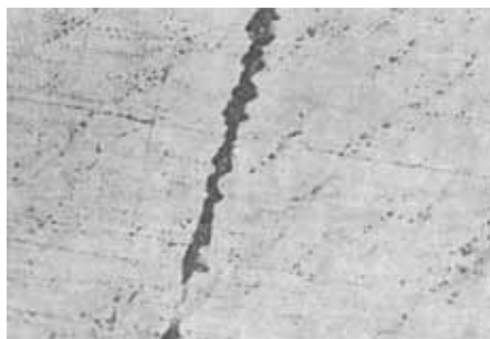
Fig. 4. A view of a small angle boundary in the (001) cleavage plane of a Nd:CaWO 4 single crystal plate. Magnification 270 \times .
