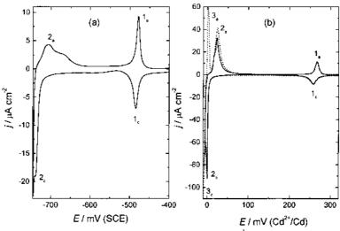
Fig. 4. Cyclic voltammograms recorded at a sweep rate of 10 mV s<sup>-1</sup> onto the (111) face of copper in a solution of 0.1 M NaCl + 0.001 M HCl + 0.005 M CdCl<sub>2</sub> (a) and 0.1 M NaCl + 0.001 M HCl + 0.01 M CdCl<sub>2</sub> (b) .
