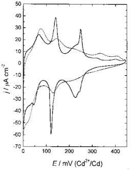
Fig. 10. Cyclic voltammograms recorded at a sweep rate of 10 mV s<sup>-1</sup> onto the (110) face of copper in a solution of 0.1 M NaCl + 0.001 M HCl + 0.1 M CdCl<sub>2</sub> before (full line) and after alloying of Cu(110) with Cd (dotted line).
