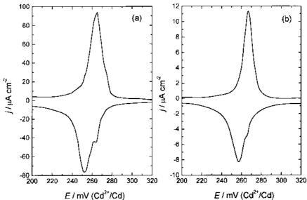
Fig. 2. Cyclic voltammograms recorded at a sweep rate of 10 mV s<sup>-1</sup> (a) and 1 mV s<sup>-1</sup> (b) onto the (111) face of copper in a solution of 0.1 M NaCl + 0.001 M HCl + 0.1 M CdCl<sub>2</sub>.
