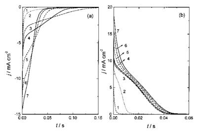
Fig. 6. Catodic potentiostatic *j*-*t* transients recorded onto the (1110 face of copper in a solution of 0.1 M NaCl + 0.001 M HCl + 0.1 M CdCl<sub>2</sub> by pulsing from  $E_{in}$ =400 mV vs. Cd<sup>2+</sup>/Cd to the following potentials (given in mV vs. Cd<sup>2+</sup>/Cd): 1.300; 2.260; 3.220; 4.200; 5.150; 6.100; 7.50. (b) Anodic *j*-*t* transients recorded by pulsing back to  $E_{in}$ .
