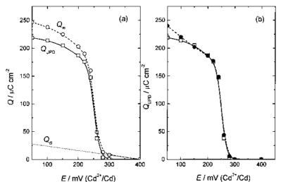
Fig. 7. (a) Q-E dependences obtained by the integration of the cathodic j-t transients shown in Fig. 6. (b) Cathodic (full line  $-\Box$ ) and anodic (dashed line  $-\bullet$ ) QUPD -E dependences obtained by integration of the cathodic and anodic j-t transients shown in Fig. 6.
