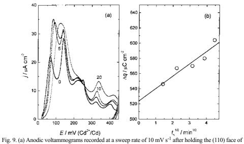
Fig. 9. (a) Anodic voltammograms recorded at a sweep rate of 10 mV s<sup>-1</sup> after holding the (110) face of copper at a potential of  $E_{\rm h} = 20$  mV vs. Cd<sup>2+</sup>/Cd for different times (marked in the Figure in minutes) in a solution of 0.1 M NaCl + 0.001 M HCl + 0.1 M CdCl<sub>2</sub>. (b) Corresponding  $q - t_{\rm h}^{1/2}$  dependences.
