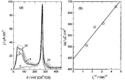
Fig. 5. (a) Anodic voltammograms recorded at a sweep rate of 10 mV s<sup>-1</sup> after holding the (111) face of copper at a potential of  $E_{\rm h} = 0$  mV vs. Cd<sup>2+</sup>/Cd for different times (marked in the Figure in minutes) in a solution of 0.1 M NaCl + 0.001 M HCl + 0.1 M CdCl<sub>2</sub>. (b) Corresponding  $q - t_{\rm h}^{1/2}$  dependences.
