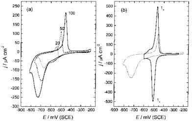
Fig. 1. (a) Cyclic voltammograms recorded at different sweep rates (marked in the figure in mV s<sup>-1</sup>) onto the (111) face of copper in a solution of 0.1 M Na Cl + 0.001 M HCl. (b) Cyclic voltammograms recorded at sweep rate of 100 mV s-1 onto the (111) copper in a solution of 0.1 M NaCl + 0.001 M HCl (dotted line) and in a solution of 0.1 M Na Cl + 0.001 M HCl + 0.005 M CdCl<sub>2</sub>
